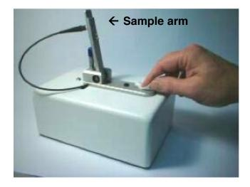
4. Pipette 2 μl of ddH2O onto the measurement pedestal, as shown in the picture.
